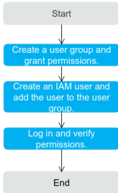
Figure 2-1 Process of granting DCS permissions
